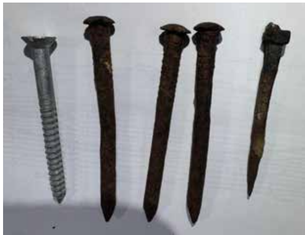
Examples of plank fasteners: Replacement #18 x 3/16" galvanized screw, and original iron spikes
